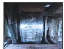
Completed RPR's with pattern welding
